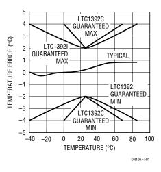
Figure 1. Output Temperature Error
